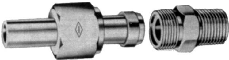
Figure 14-1 An assembly in which a sleeve is brazed to the tubing, and the nut is then screwed onto the fitting.
