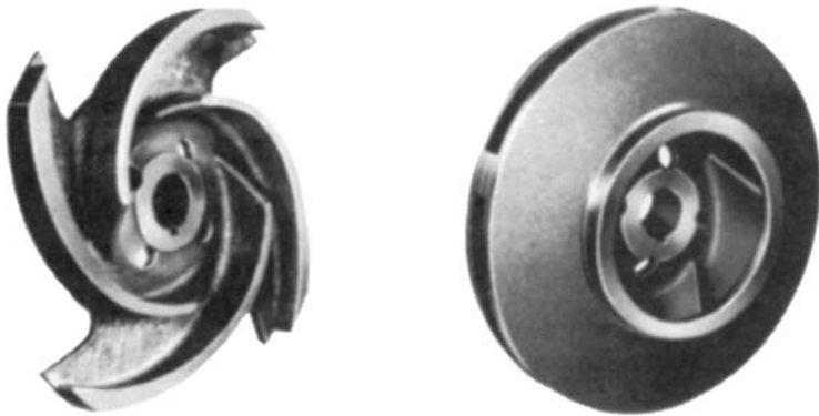
Figure 3-19 Open-type (left) and enclosed-type (right) impellers.
