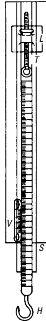
Figure 2-24 Hook gage, used to measure the depth of water above a weir.
