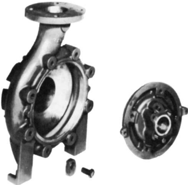
Figure 3-18 An offset-volute design of casing (left) and cover (right). The casing is designed for top centerline discharge, self-venting, and back pullout. (Courtesy Buffalo Forge Company)
