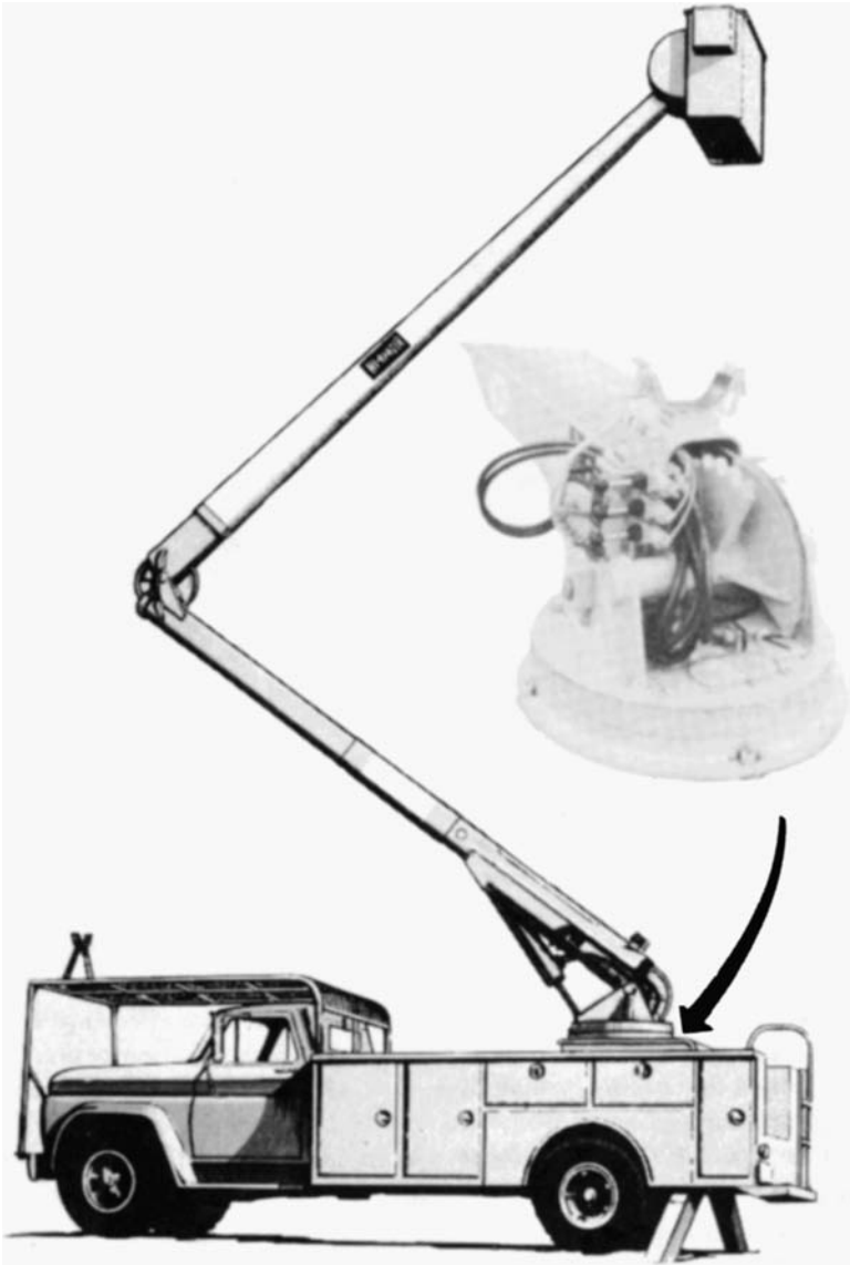
Figure 9-1 Aerial towers with hydraulic actuation are used by utility companies and fire departments. (Courtesy Mobile Aerial Towers, Inc.)
