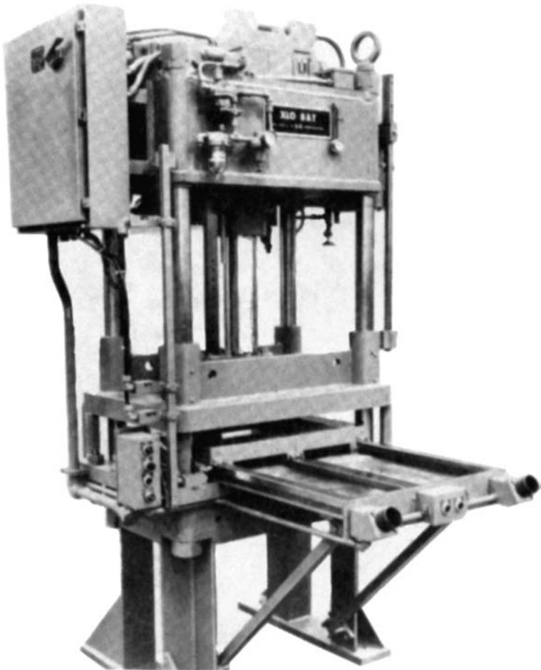
Figure 9-3 A 28-ton hydraulic trim press.
