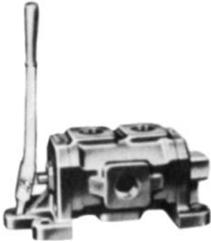
Figure 12-6 A hydraulic directional control valve with a hand-type operator.
