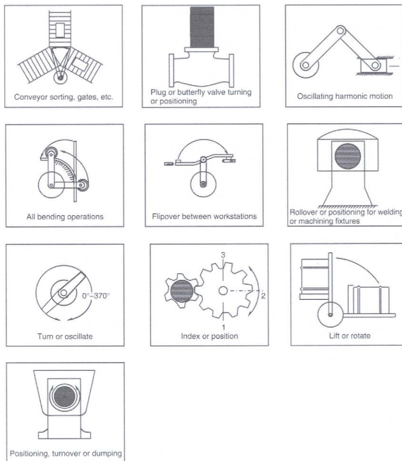
Figure 4.2 Application of limited rotation hydraulic motor
