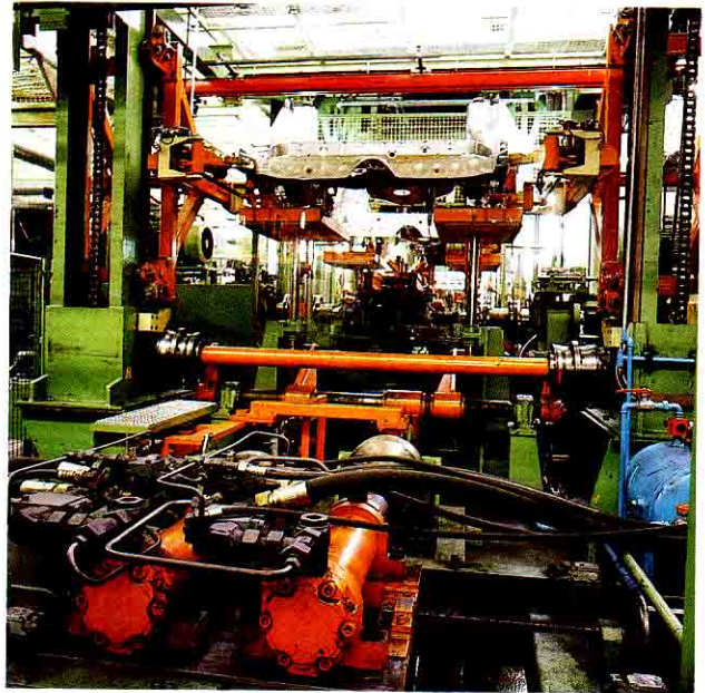
Fig. 2: One cylinder (at top) - the other one being used as a standby device - moves all stations simultaneously in conjunction with a lifting mechanism.
