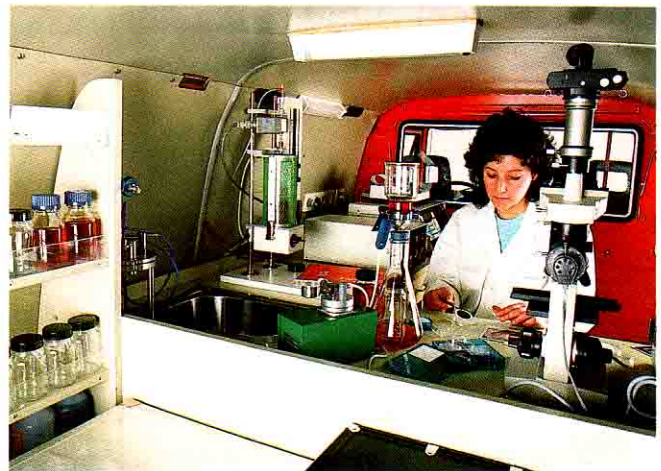
Fig. 267: Mobile laboratory for on-site analysis
