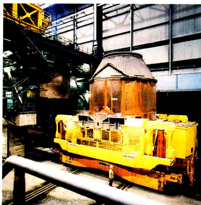
Fig. 277: Vessel changing vehicle is moved into position via the rail crossing point
