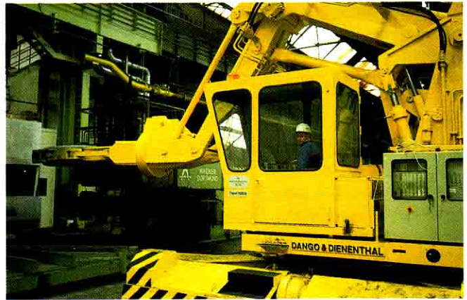
Fig. 34: Mobile manipulator in operation
