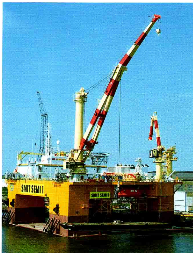
Fig. 42: 700 kW crane installation on a semi-submersible.
