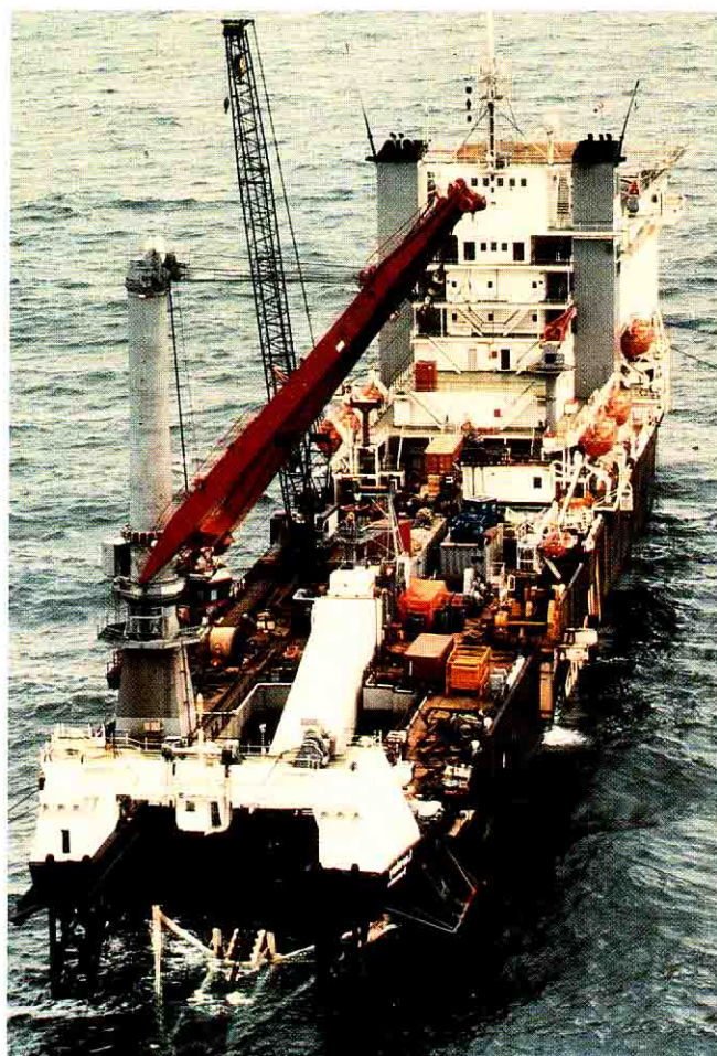
Fig. 41: 3000 kN tower crane on a pipe layer
