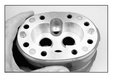
**4** Install new *seal* and new *backup gasket* into wear plate. Note in the middle of the backup gasket a flat section or support. This area must face away from the wear plate inside the seal.
