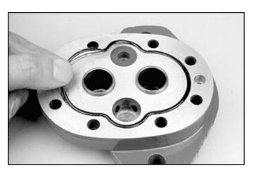
**3** Apply a thin coat of petroleum jelly or hydraulic oil to both milled gear pockets of body. Slip body onto front plate with half moon port cavities in body facing away from front plate.
