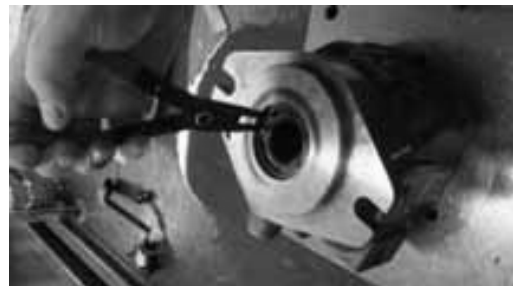
24. Remove Shaft Seal With the seal retaining ring removed use a punch or similar tool to knock out the shaft seal.
