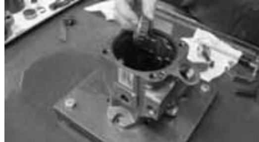
22. Remove Cradle Bearings Note: The cradle bearings are asymmetrical. Note proper orientation shown in picture.
