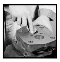
2) If the bushings have been removed, deburr the bushing bores with an emery cloth. Rinse parts in a solvent. Air blast all the parts and wipe with a clean, lintless cloth before starting assembly.
