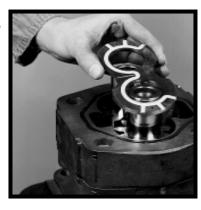
16) Slip the thrust plate with the seal over the gear journals and into the housing bore. The flat side of the seal should face up with the relief groove facing the outlet side. (For single pump assemblies go directly to Step #21).
