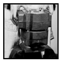
7) Carefully lift or pry off the bearing carrier to prevent damage to contact face and edges. Dowel pins will remain in either the bearing carrier or the gear housing. DO NOT REMOVE THEM. For multiple assemblies only
