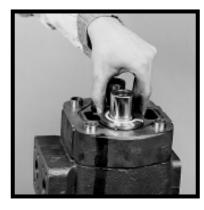
**4)** Remove the thrust plate. Examine and replace if necessary. See wear guide page 10.
