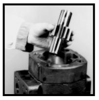
**19)** Place the thrust plate in the gear housing per Step #14. Insert the drive and driven gears of the second section in their respective bearings. Make certain the gears are in contact with the thrust plate face. Place the port end cover plate in the housing per Step #16. For multiple assemblies only
