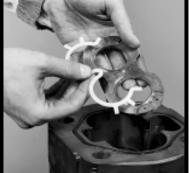
13) Assemble the channel seals into the grooves in the thrust plates with the flat side of the seal facing away from the thrust plate as shown below.
