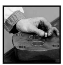
20) Check the plug or plugs in the port end cover to be sure that they are tight. Follow the procedure outlined in Step #4 for new plugs. For multiple assemblies only
