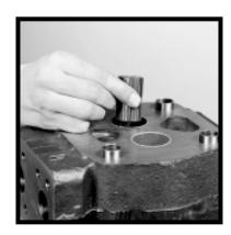
18) Insert the connecting shaft into the spline of the drive gear. Position and place the second gear housing on the bearing carrier as outlined in Step #12. For multiple assemblies only
