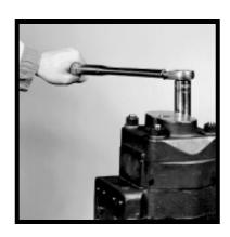
2) Use a socket wrench to remove the 4 cap screws on single units or the 4 hex nuts, studs and washers of multiple units.
