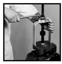
Use a bushing puller as shown in the tool list to remove bushings (see page 4).
