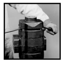
3) Lift off the port end cover. If prying is necessary, be careful not to damage the machined surfaces. Dowel pins will remain in either the port end cover or the gear housing.
