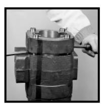
6) Lift the gear housing from the bearing carrier. If prying is necessary, take care not to damage machined surfaces. Examine and replace if necessary. (See page 10) For multiple assemblies only
