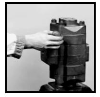
1) Place the pump in a vise with the drive shaft pointIng down. Caution: DO NOT GRIP ON OR NEAR ANY MACHINED SURFACES DURING ASSEMBLY OR DISASSEMBLY. Match-mark all sections. Be sure to align these marks when reassembling.
