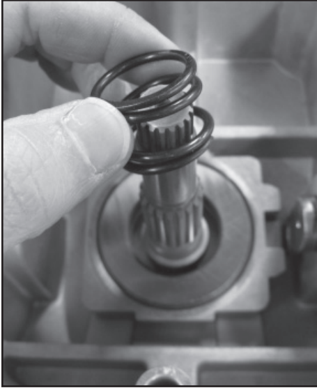
Install central spring into rear housing
