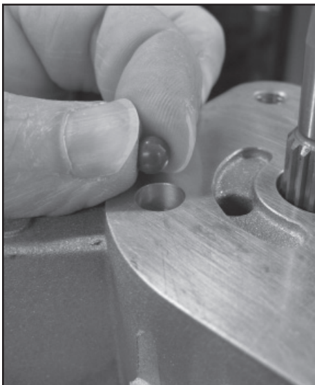
Install charge relief ball
