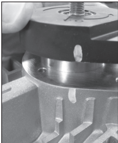
Align charge cover with marks
