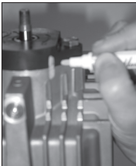
Mark charge pump cover to housing
