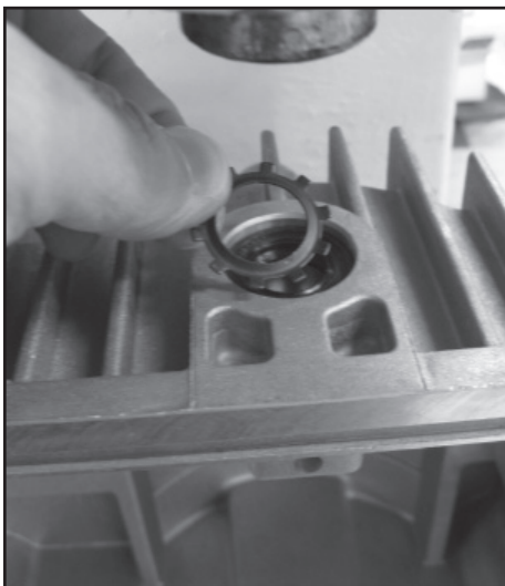
Press in seal retainers
