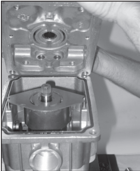
Remove center block and rear housing
