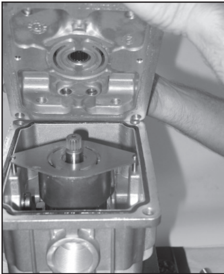
Align center block to front housing
