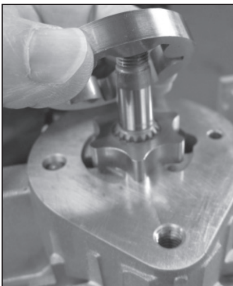
Lift off charge pump rotor set
