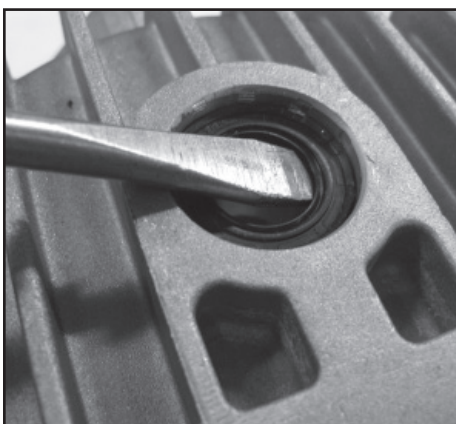
Trunnion seal removal
