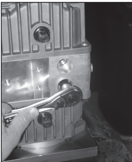
Check /shock valve removal
