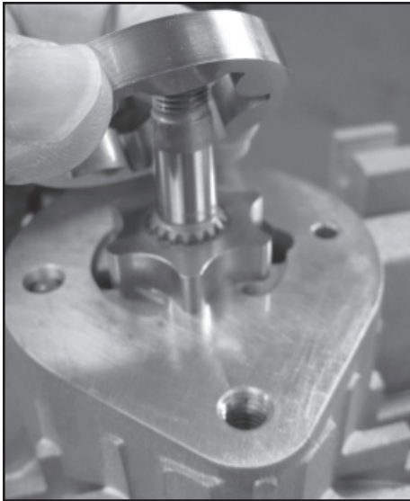
Install charge rotor set
